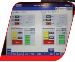
Sample Co-Extruder screen used in blow molding containers on a high-speed container line. Note complexity of multi-stage operation including upstream and downstream equipment plus trimming equipment.
